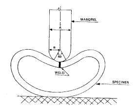
The reverse bend test shall be carried out with a mandrel. Radius (R) and width (A) of mandrel shall be calculated for any combination of diameter, wall thickness and grade with the formula.
