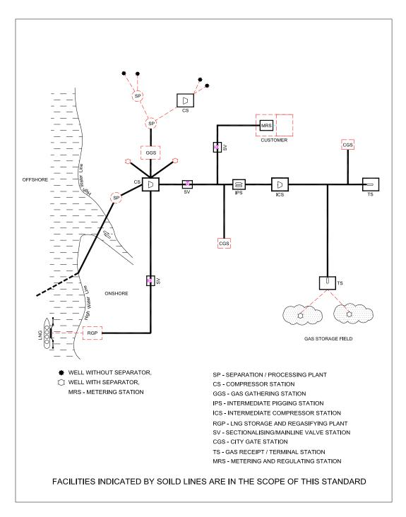
**Note:** Subsea pipeline for transportation of gas after its primary treatment stations or gas gathering stations shall also be included in the scope of the standard.
